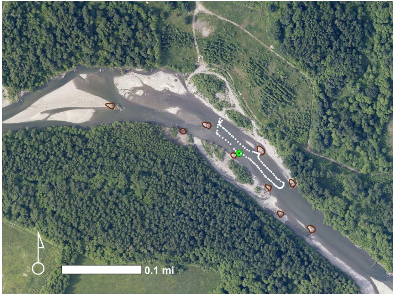
Figure 104: Digital temperature sensor cable lay-out in the Downstream of Hutchinson Project reach. Green point shows location of anomaly at 320m shown in Figure 105 (Gendaszek 2014).
