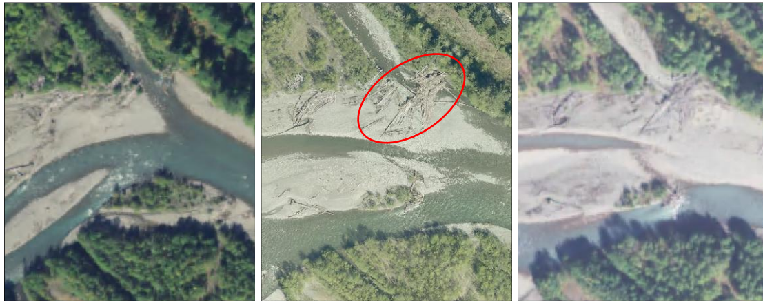
Figure 42: Channel change at the head of the target side channel between logjam #1 and #2 (left: 2015, center: 2016, right: 2017).
