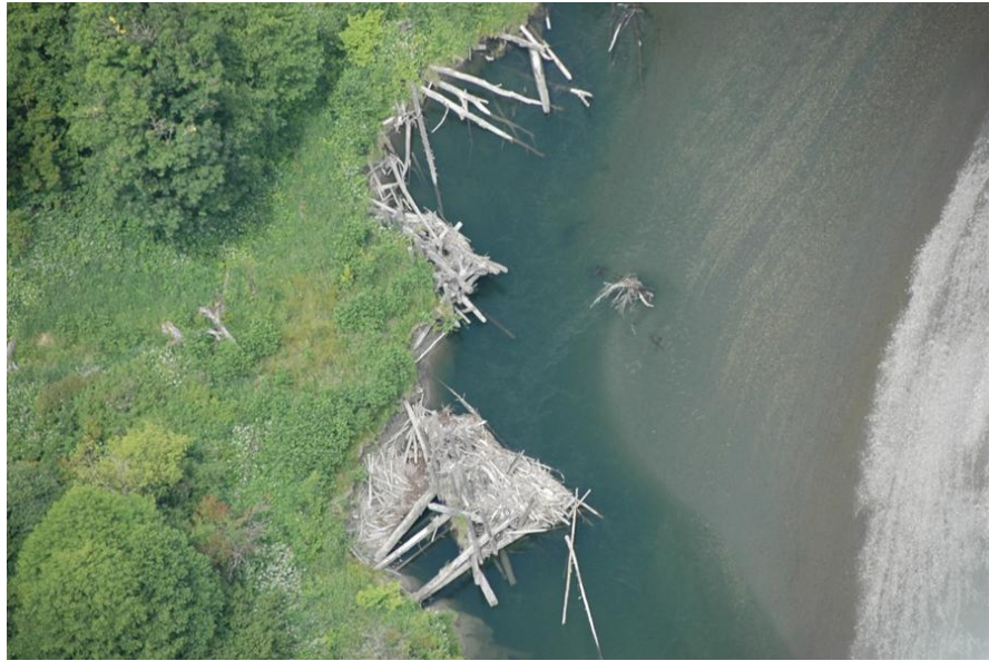
Figure 134: Aerial view of pool-formation associated with engineered logjams (#8 and #9) (June 2014).
