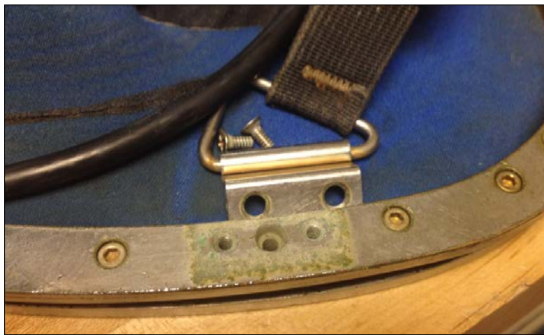
Neck ring screws missing from beneath chin strap retainers
