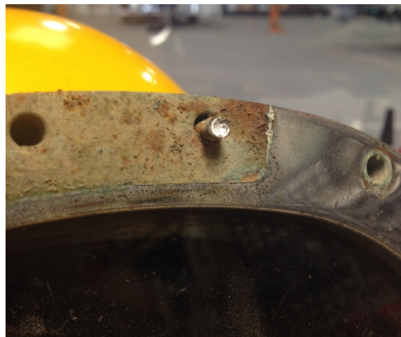
Several face-port screws seized; one had to be drilled for removal
