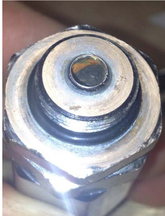
Damaged inlet knife-edge; does not seal properly
