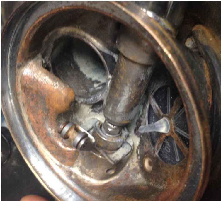
Mud in regulator, old nut, worn soft seat, and regulator not serviced
