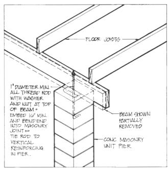
Figure 4.37. Masonry Pier-Bolt Through Beam
