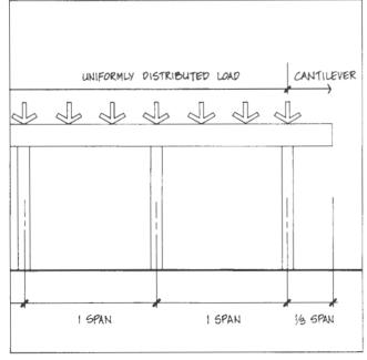
Figure 4.39. Floor Beam with Cantilever Overhang
