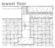
Figure 1.3. Elevation Requirements for Slab Foundations
