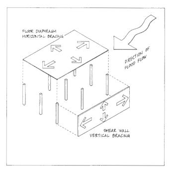
Figure 4.25. Floor Diaphragm Bracing
