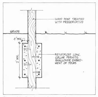
Figure 4.5. Reinforced Concrete Collar
