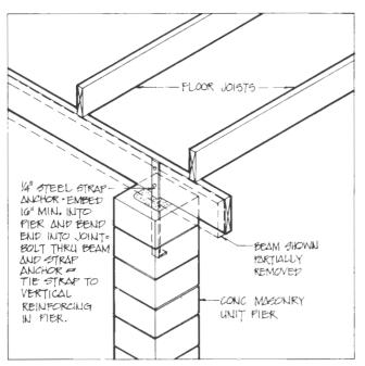
Figure 4.36. Masonry Pier—Strap Anchor
