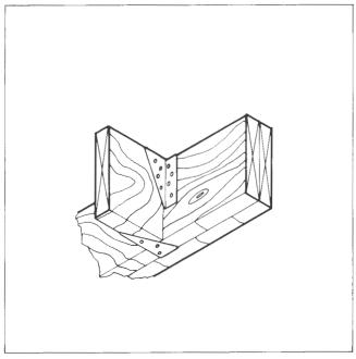
Figure 4.27. Metal Framing Anchors
