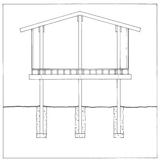
Figure 4.29. Pole Frame Construction
