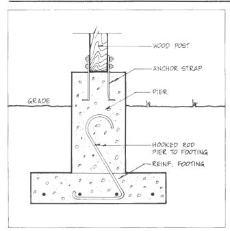
Figure 4.9. Post/Pier Foundation
