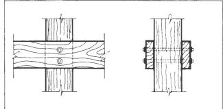
Figure 4.31. Bolted Connection to Round Pole
