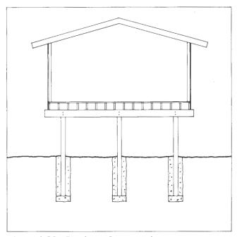
Figure 4.28. Platform Construction
