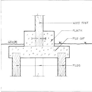
Figure 4.8. Post/Pile Foundation
