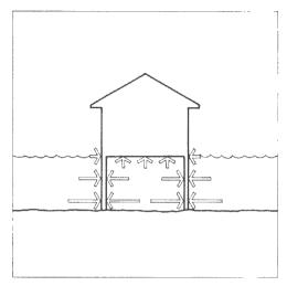
Figure 2.1. Hydrostatic Forces
