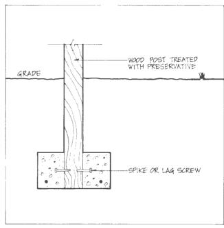
Figure 4.11. Spike Anchorage of Post
