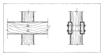
Figure 4.33. Dapped Pole Connection
