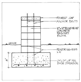
Figure 4.17. Reinforced Concrete Masonry Pier
