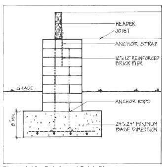
Figure 4.16. Reinforced Brick Pier
