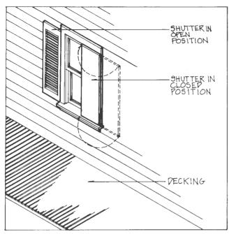
Figure 4.47. Shutters for Window Protection
