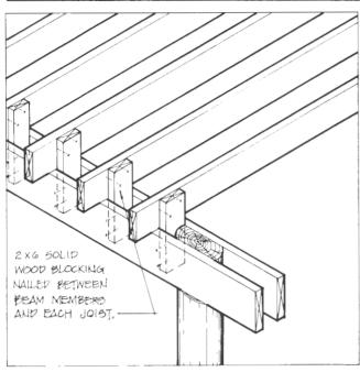
Figure 4.41. Wood Joist Anchors
