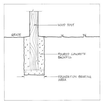
Figure 4.7. Post on Concrete Bearing Pad
