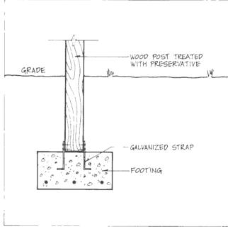
Figure 4.13. Galvanized Strap Anchorage Detail
