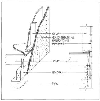
Figure 4.45. Plywood Anchorage
