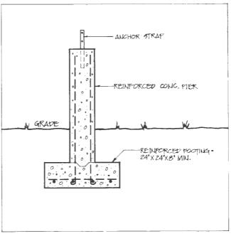
Figure 4.19. Reinforced Concrete Pier
