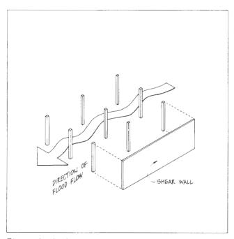
Figure 4.24. Shear Wall Bracing
