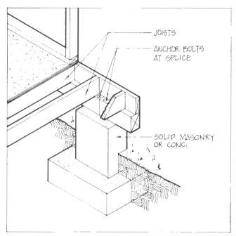
Figure 4.38. Beam Splice on Pier
