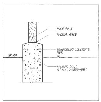
Figure 4.12. Metal Angle Anchorage Detail
