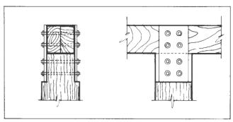
Figure 4.32. Dapped Gusset Plate Connection
