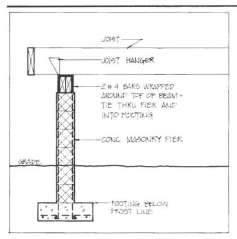
Figure 4.35. Concrete Masonry Unit Pier
