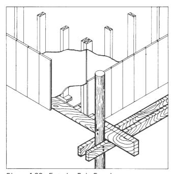
Figure 4.30. Exterior Pole Framing
