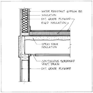
Figure 4.52. Insulated Floor Section, Foundation Wall
