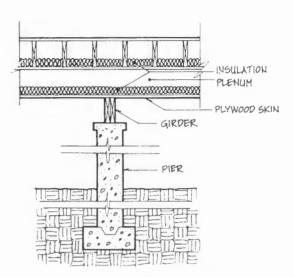
Figure 4.53. Double-Insulated Floor Plenum, Pier Foundation
