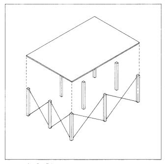
Figure 4.22. Diagonal Bracing
