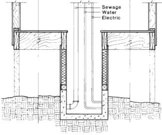
Figure 4.48. Protective Utility Shaft
