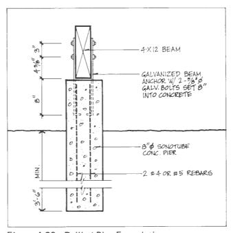
Figure 4.20. Drilled Pier Foundation
