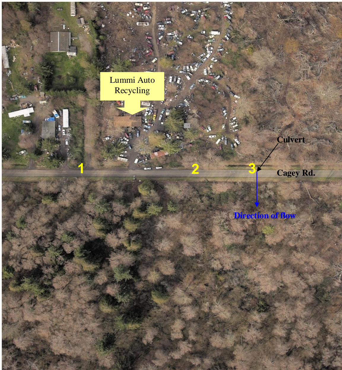
Figure 1. Sampling locations along the ditch adjacent to the Lummi Auto Recycling. The samples were taken from the ditch on the north side of Cagey Road just upstream (1), immediately downstream (2), and further downstream (3) of Lummi Auto Recycling
