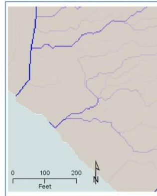
Figure 2. A typical flow accumulation surface; each cell stores the count of cells that pour into that cell. Higher cell counts are displayed as a darker blue. Coloration does not necessarily indicate a perennial or seasonal stream.
