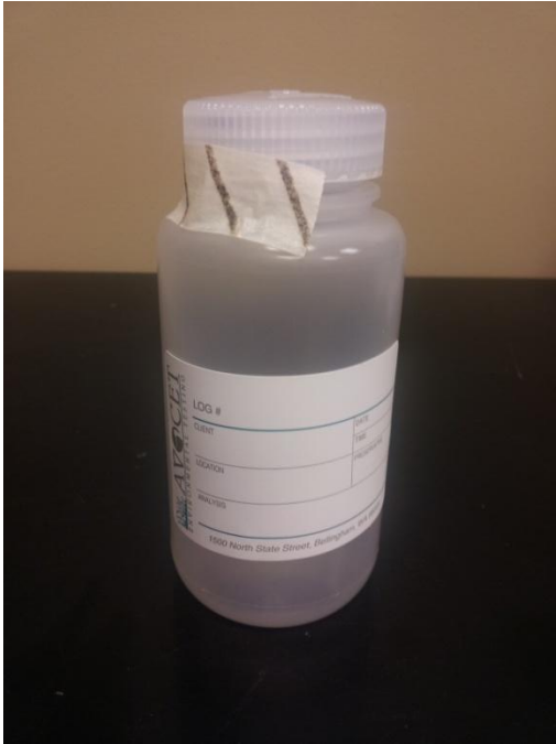
Figure 2.1 Example of Bacteria Sample Bottle Provided by Edge Analytical with Autoclave Tape Across Side of Lid
