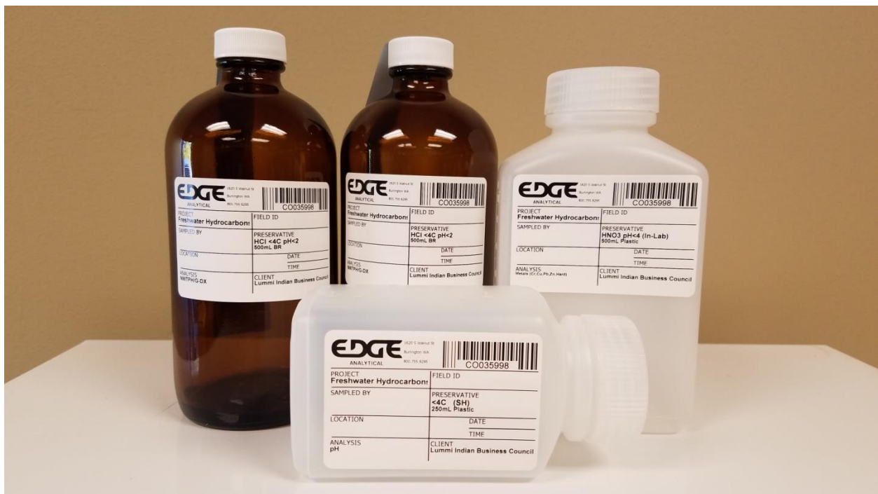
Figure 2.2 Example of Bottles for Collection of Metal and Hydrocarbon Samples
