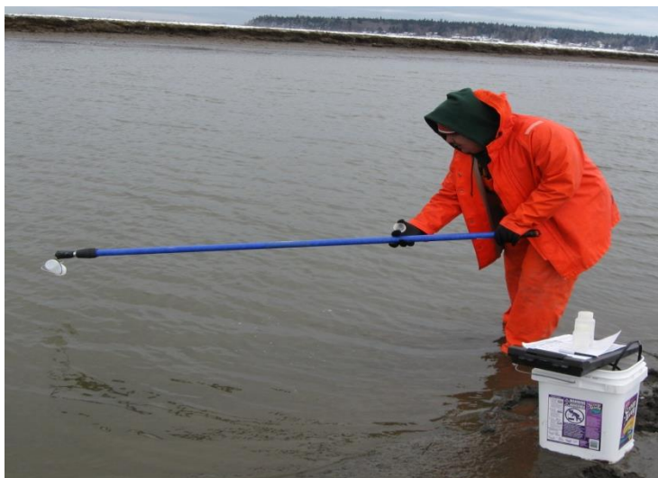
Figure 3.1 TOC Sample Collection Using a Sampling Wand
