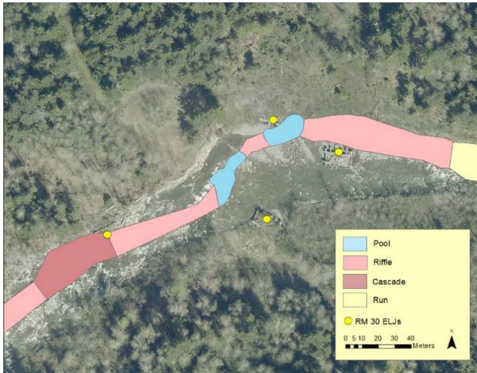
Figure 7. Channel unit map for the River Mile 30 project reach from the 2005 field surveys. (LNR 2005 data, photo from 2016, Source: NNR and LNR 2019).
