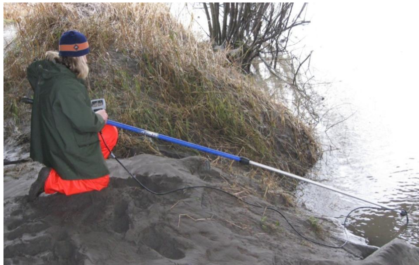
Figure 4.1 Surface Water Quality Sample Collection Using a Sampling Wand
