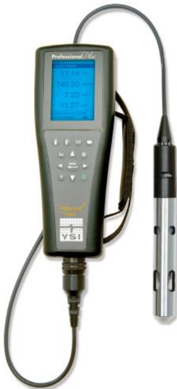
Figure 2.1 Photo of YSI ProPlus Showing Hand-Held Instrument, Cable, and Sonde (note that probe guard of actual unit is a different type)
